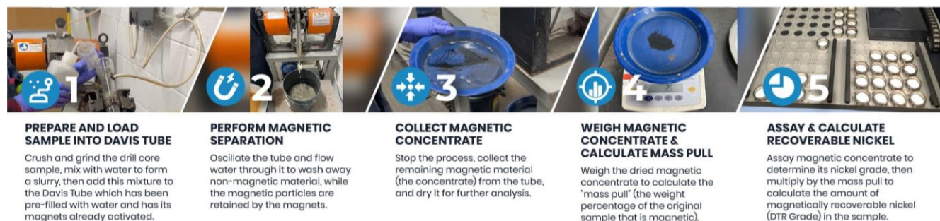
Figure 11: Davis Tube Recovery (DTR) Metallurgical Test 5 Step Process
