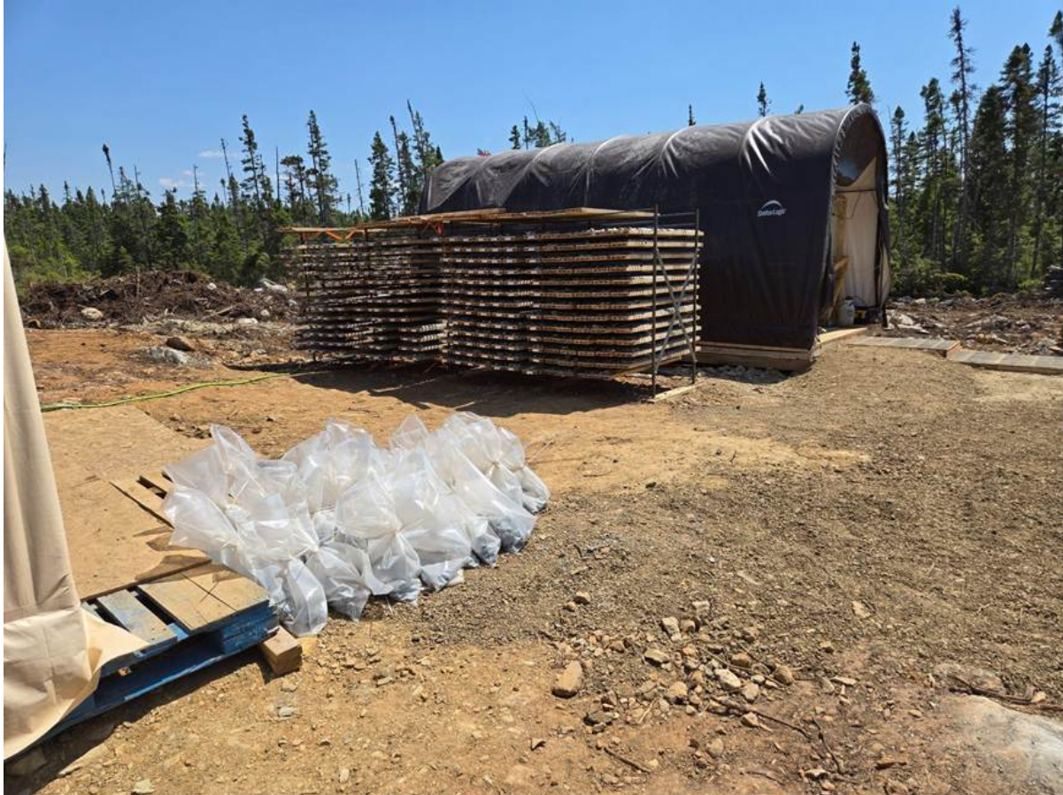
Figure 2: Drill Core from RPM Phase 2X Program preparing for shipment to analytical lab for assay & Davis Tube metallurgical testing
