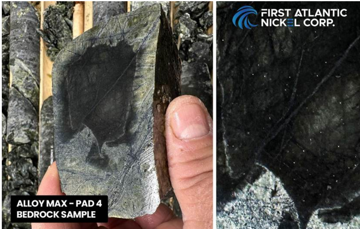
Figure 01: Bedrock sample collected beneath shallow overburden at a drill pad location. The sample confirms the drill target prior to drilling and contains visible disseminated awaruite magnetic nickel cobalt alloy mineralization.
