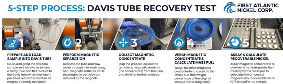
Figure 6: Davis Tube Recovery (DTR) Metallurgical Test 5 Step Process
